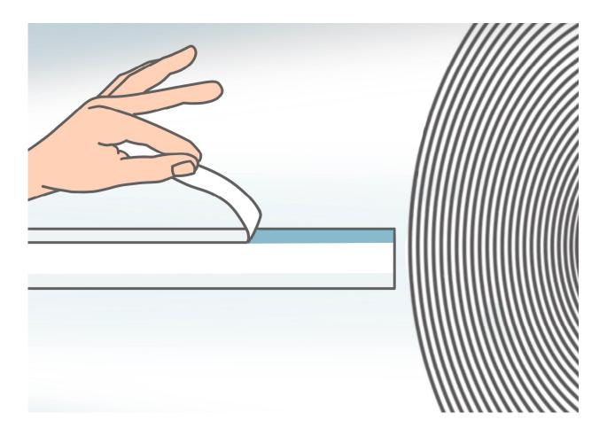
Remove the narrow part of the liner of Splice tape
