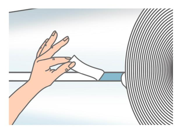
Remove the other part of liner of Splice tape
