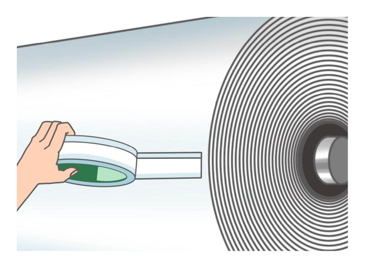
Apply the Splice tape along the tube axis
